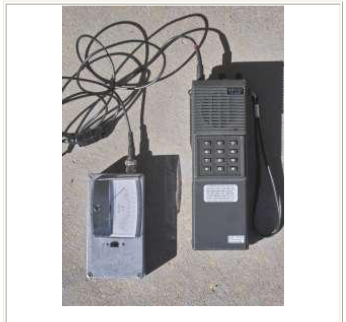
Figure 1: The Field Strength Meter (Mark II) and interconnect cable with the modified Icom IC-2A/T
