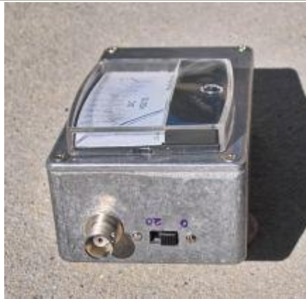
Figure 3: A close-up of the top of the unit showing the input connector and switchable 20 dB attenuator .
