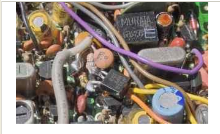
Figure 2 (top) and Figure 3 (bottom): Two different view of the JFET buffer circuit tacked atop IC1.
