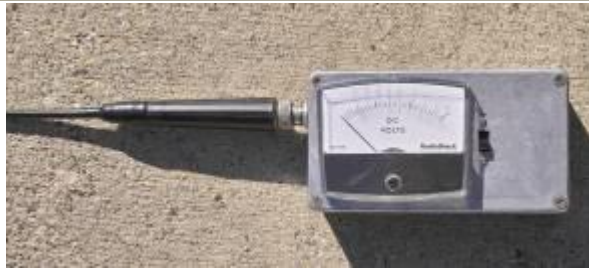
Figure 1: The as-built prototype of the "Mark II" field strength meter.
