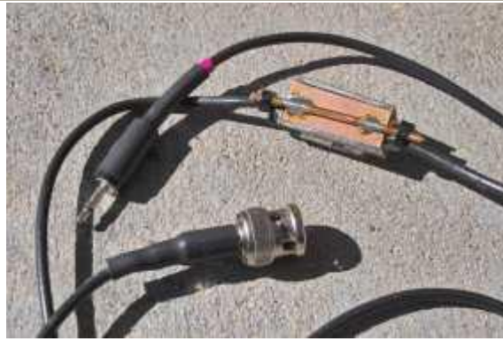
Figure 6: A close-up of the interconnect cable and the 10.7 MHz bandpass filter. The circuit was constructed in a small enclosure made of circuit board material and a piece of #12 wire was soldered to it, providing an anchor point for the strain reliefs on the coax.
