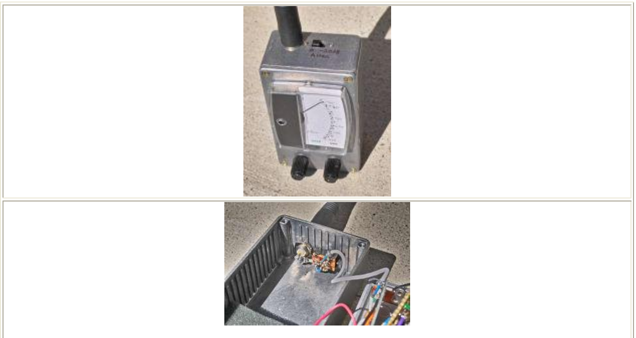
Figure 4: Top: The top view of the field-strength meter showing the antenna connection and the attenuator switch. Bottom: This shows the components of the 20 dB attenuator. (Yes, I know that it says "-20 dB" attenuation...)
