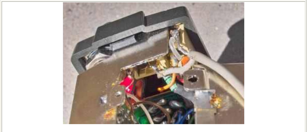
Figure 4 (top): Overview of the inside of the modified IC-2A/T showing the connection to the buffer circuit and cable routing.
