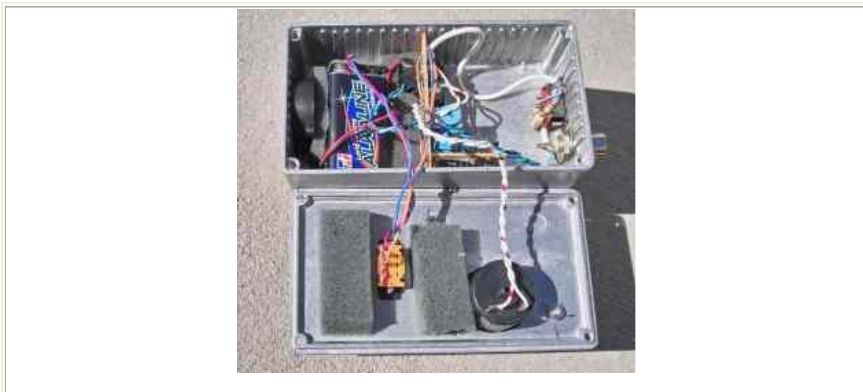
Figure 2: Inside the field strength meter, showing the placement of the circuit board, battery, piezoelectric speaker, RF connector, and switches.
